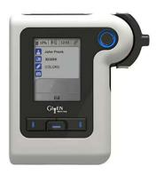
The PillCam<sup>™</sup> recorder is a recording device with a built in real-time viewer, which is worn by the patient during the PillCam<sup>™</sup> procedure. Following the procedure, the physician downloads the images from the PillCam<sup>™</sup> recorder for interpretation.
